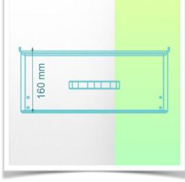
Mechanical data Internal dimensions 420 x 397 x 160 mm
