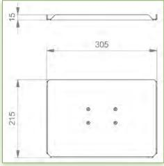
Display Compatibility: 26" Wide ( Weight) Supported Weight: 4- 9,5 Kg VESA standard: 75 / 100 mm Keyboard-Mouse holder: 300 x 210 mm
