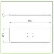
Display Compatibility: 26" Wide ( Weight) Supported Weight: 12,5 Kg VESA standard: 75 / 100 mm Keyboard-Mouse holder: 580 x 200 mm
