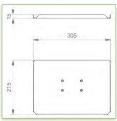
Display Compatibility: 26" Wide ( Weight) Supported Weight: 3- 7 Kg VESA standard: 75 / 100 mm Keyboard-Mouse holder: 300 x 210 mm
