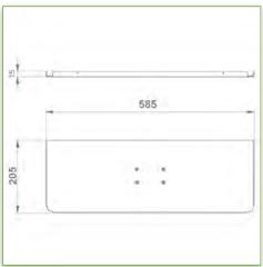
Display Compatibility: 26" Wide ( Weight) Supported Weight: 15 Kg VESA standard: 75 / 100 mm Keyboard-Mouse holder: 580 x 200 mm
