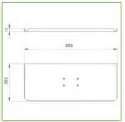
Display Compatibility: 26" Wide ( Weight) Supported Weight: 4- 9,5 Kg VESA standard: 75 / 100 mm Keyboard-Mouse holder: 500 x 200 mm
