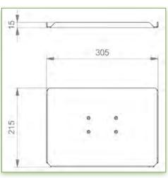
Display Compatibility: 26" Wide ( Weight) Supported Weight: 15 Kg VESA standard: 75 / 100 mm Keyboard-Mouse holder: 300 x 210 mm
