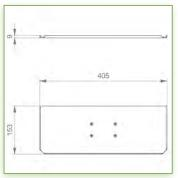
Display Compatibility: 26" Wide ( Weight) Supported Weight: 3-7 Kg VESA standard: 75 / 100 mm Keyboard-Mouse holder: 400 x 150 mm
