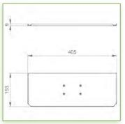
Display Compatibility: 26" Wide ( Weight) Supported Weight: 4- 9,5 Kg VESA standard: 75 / 100 mm Keyboard-Mouse holder: 400 x 150 mm
