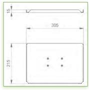
Display Compatibility: 26" Wide ( Weight) Supported Weight: 11- 15,5 Kg VESA standard: 75 / 100 mm Keyboard-Mouse holder: 300 x 210 mm
