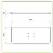
Display Compatibility: 26" Wide ( Weight) Supported Weight: 2-4,5 Kg VESA standard: 75 / 100 mm Keyboard-Mouse holder: 500 x 200 mm
