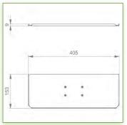
Display Compatibility: 26" Wide ( Weight) Supported Weight: 11- 15,5 Kg VESA standard: 75 / 100 mm Keyboard-Mouse holder: 400 x 150 mm
