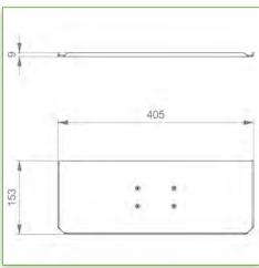
Display Compatibility: 26" Wide (Weight) Supported Weight: 11- 15,5 Kg VESA standard: 75 / 100 mm Keyboard-Mouse holder: 400 x 150 mm
