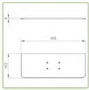
Display Compatibility: 26" Wide ( Weight) Supported Weight: 12,5 Kg VESA standard: 75 / 100 mm Keyboard-Mouse holder: 400 x 150 mm
