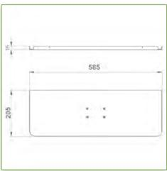
Display Compatibility: 26" Wide ( Weight) Supported Weight: 12,5 Kg VESA standard: 75 / 100 mm Keyboard-Mouse holder: 580 x 200 mm
