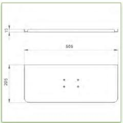
Display Compatibility: 26" Wide ( Weight) Supported Weight: 3- 7 Kg VESA standard: 75 / 100 mm Keyboard-Mouse holder: 500 x 200 mm
