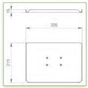
Display Compatibility: 26" Wide ( Weight) Supported Weight: 3-7 Kg VESA standard: 75 / 100 mm Keyboard-Mouse holder: 300 x 210 mm
