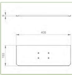
Display Compatibility: 26" Wide ( Weight) Supported Weight: 12,5 Kg VESA standard: 75 / 100 mm Keyboard-Mouse holder: 400 x 150 mm
