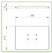
Display Compatibility: 26" Wide ( Weight) Supported Weight: 15 Kg VESA standard: 75 / 100 mm Keyboard-Mouse holder: 300 x 210 mm
