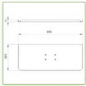
Display Compatibility: 26" Wide ( Weight) Supported Weight: 12,5 Kg VESA standard: 75 / 100 mm Keyboard-Mouse holder: 500 x 200 mm
