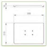
Display Compatibility: 26" Wide ( Weight) Supported Weight: 10- 11,5 Kg VESA standard: 75 / 100 mm Keyboard-Mouse holder: 300 x 210 mm
