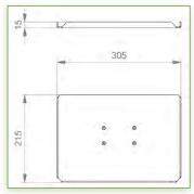
Display Compatibility: 26" Wide ( Weight) Supported Weight: 2- 4,5 Kg VESA standard: 75 / 100 mm Keyboard-Mouse holder: 300 x 210 mm
