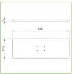
Display Compatibility: 26" Wide ( Weight) Supported Weight: 3- 7 Kg VESA standard: 75 / 100 mm Keyboard-Mouse holder: 580 x 200 mm
