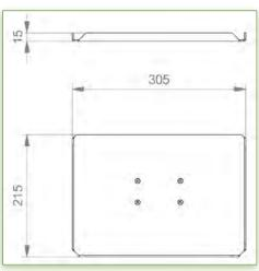
Display Compatibility: 26" Wide ( Weight) Supported Weight: 18 Kg VESA standard: 75 / 100 mm Keyboard-Mouse holder: 300 x 210 mm
