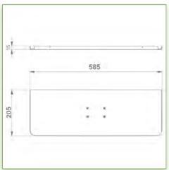
Display Compatibility: 26" Wide ( Weight) Supported Weight: 10- 11,5 Kg VESA standard: 75 / 100 mm Keyboard-Mouse holder: 580 x 200 mm
