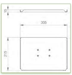
Display Compatibility: 26" Wide ( Weight) Supported Weight: 4- 9,5 Kg VESA standard: 75 / 100 mm Keyboard-Mouse holder: 300 x 210 mm
