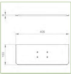
Display Compatibility: 26" Wide ( Weight) Supported Weight: 4- 9,5 Kg VESA standard: 75 / 100 mm Keyboard-Mouse holder: 400 x 150 mm
