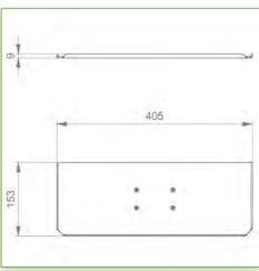
Display Compatibility: 26" Wide ( Weight) Supported Weight: 18 Kg VESA standard: 75 / 100 mm Keyboard-Mouse holder: 400 x 150 mm
