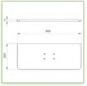
Display Compatibility: 26" Wide ( Weight) Supported Weight: 10- 11,5 Kg VESA standard: 75 / 100 mm Keyboard-Mouse holder: 500 x 200 mm
