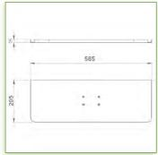
Display Compatibility: 26" Wide ( Weight) Supported Weight: 2- 4,5 Kg VESA standard: 75 / 100 mm Keyboard-Mouse holder: 580 x 200 mm
