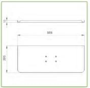
Display Compatibility: 26" Wide ( Weight) Supported Weight: 18 Kg VESA standard: 75 / 100 mm Keyboard-Mouse holder: 500 x 200 mm
