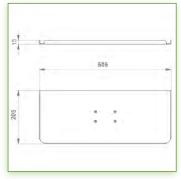
Display Compatibility: 26" Wide ( Weight) Supported Weight: 11- 15,5 Kg VESA standard: 75 / 100 mm Keyboard-Mouse holder: 500 x 200 mm
