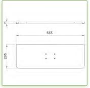
Display Compatibility: 26" Wide ( Weight) Supported Weight: 4- 9,5 Kg VESA standard: 75 / 100 mm Keyboard-Mouse holder: 580 x 200 mm
