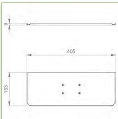
Display Compatibility: 26" Wide ( Weight) Supported Weight: 2- 4,5 Kg VESA standard: 75 / 100 mm Keyboard-Mouse holder: 400 x 150 mm
