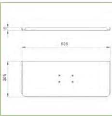
Display Compatibility: 26" Wide (Weight) Supported Weight: 18 Kg VESA standard: 75 / 100 mm Keyboard-Mouse holder: 580 x 200 mm
