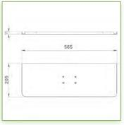
Display Compatibility: 26" Wide ( Weight) Supported Weight: 18 Kg VESA standard: 75 / 100 mm Keyboard-Mouse holder: 580 x 200 mm
