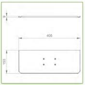
Display Compatibility: 26" Wide ( Weight) Supported Weight: 18 Kg VESA standard: 75 / 100 mm Keyboard-Mouse holder: 400 x 150 mm
