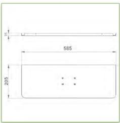
Display Compatibility: 26" Wide ( Weight) Supported Weight: 11- 15,5 Kg VESA standard: 75 / 100 mm Keyboard-Mouse holder: 580 x 200 mm
